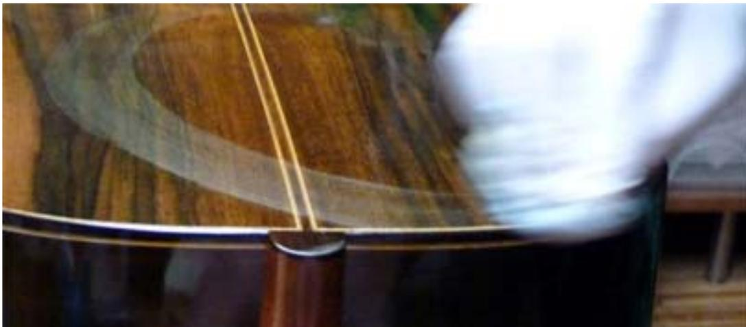
*[Application of shellac: the varnish drenched pad leaves a trail that makes a new layer in the thickness of few molecules.]*
