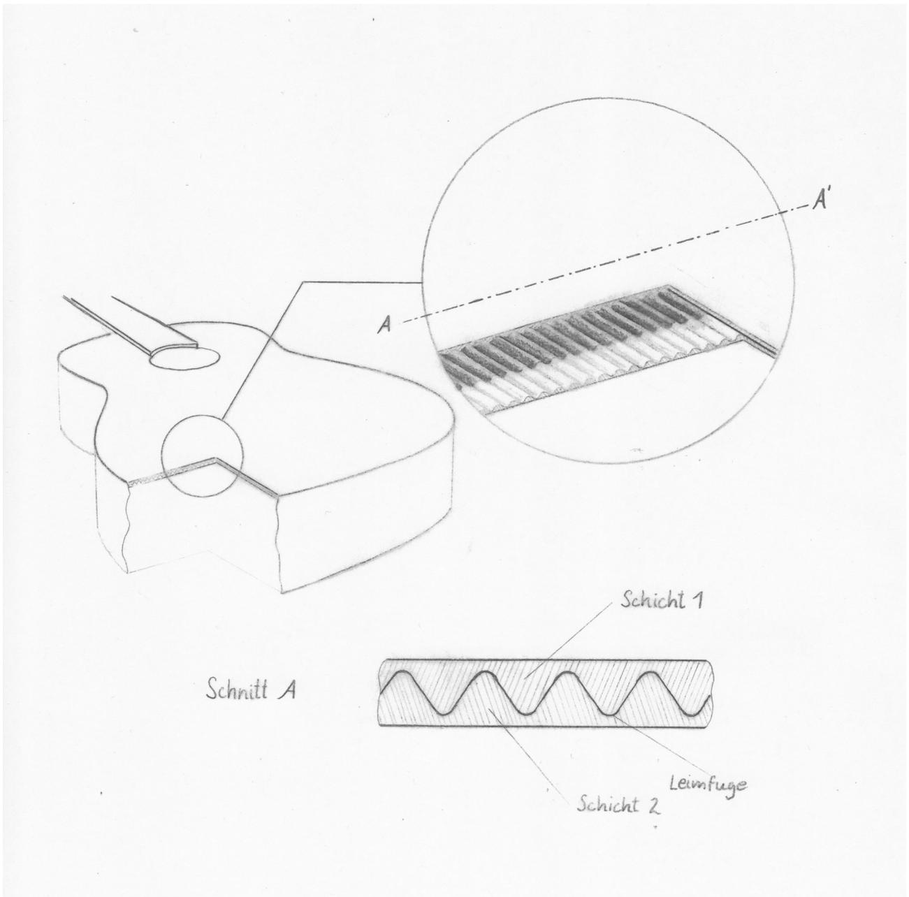
A drawing from the patent application I never filed. Any instrument maker who wants to make *Enhanced Wood* soundboards has my permission to do so on the condition of stating the origin of the idea.
